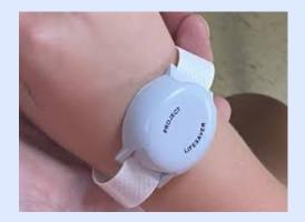
The Project Lifesaver device relies on radio technology and specially trained search and rescue teams to locate at-risk individuals who have eloped. The device is designed so it cannot be removed from an individual's wrist or ankle to provide 24/7 monitoring. This device is maintained and monitored by police.
